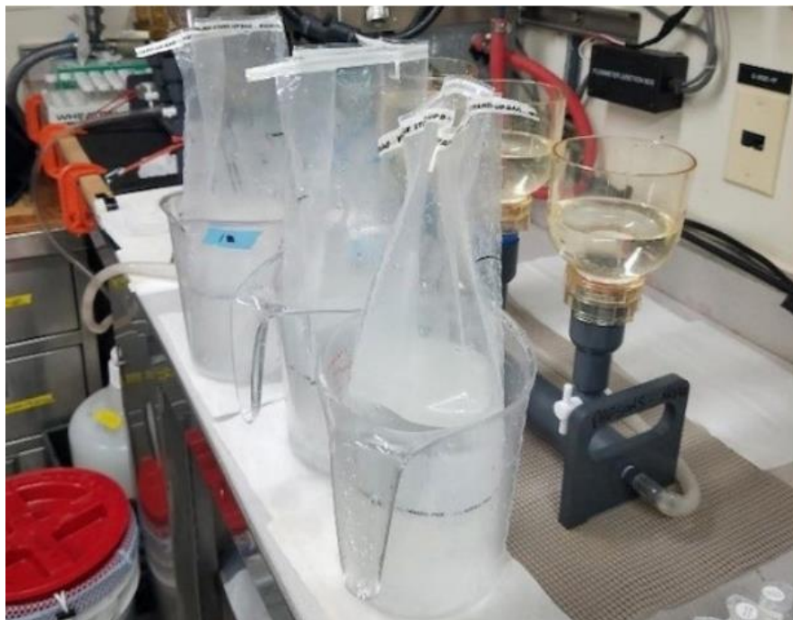
Figure 2 eDNA detection operation experiment (Adapted from Douglas et al., 2020)
